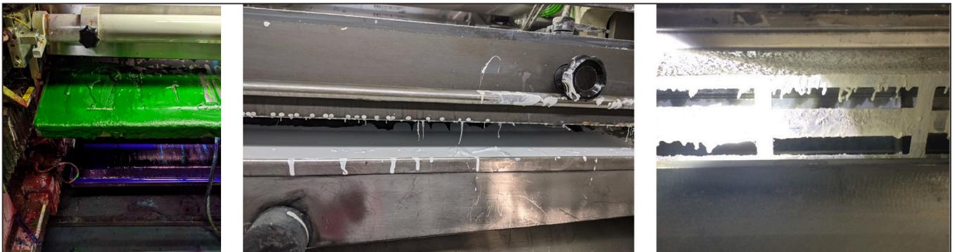
Back doctoring is a condition where returning ink is prevented from re-entering a chamber, because the containment blade is too stiff. As a result, ink falls into the drip pan resulting in thousands of gallons of ink wasted each week. Often, it's necessary to stop the press mid-run. Changing to a 0.006-in. radius blade and reducing pump pressure completely eliminates back-doctoring.
